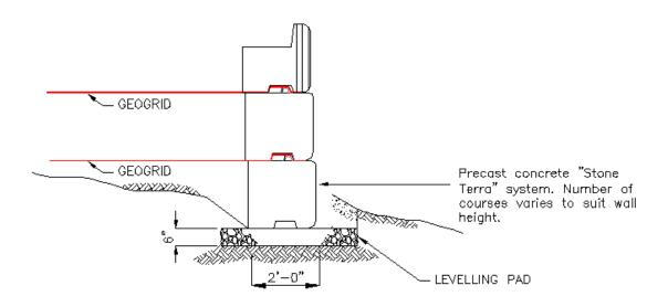
**NOTE:** Take care to align the grid properly to the wall so that the strength direction of the grid is perpendicular to the wall face. Generally, the grid will be rolled back from the blocks (behind the face of the wall) and cut to the proper reinforcement length. *In other words, grid cannot be rolled along the length of the wall, parallel to the wall face.* Check with your grid manufacturer if you are unsure about proper grid installation.
